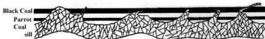
Section of Sill in the workings of the Panny Pit, Kirkcaldy (Communicated by Messrs. Herd, Dunnikier Colliery)
