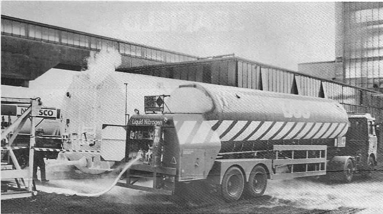
A supply of nitrogen is delivered and stored as part of the drive to prevent heatings
